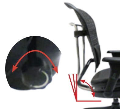
Backrest Tilt Tension Adjustment Twist knob under seat to adjust backrest tension. Twisting clockwise increases tension.
